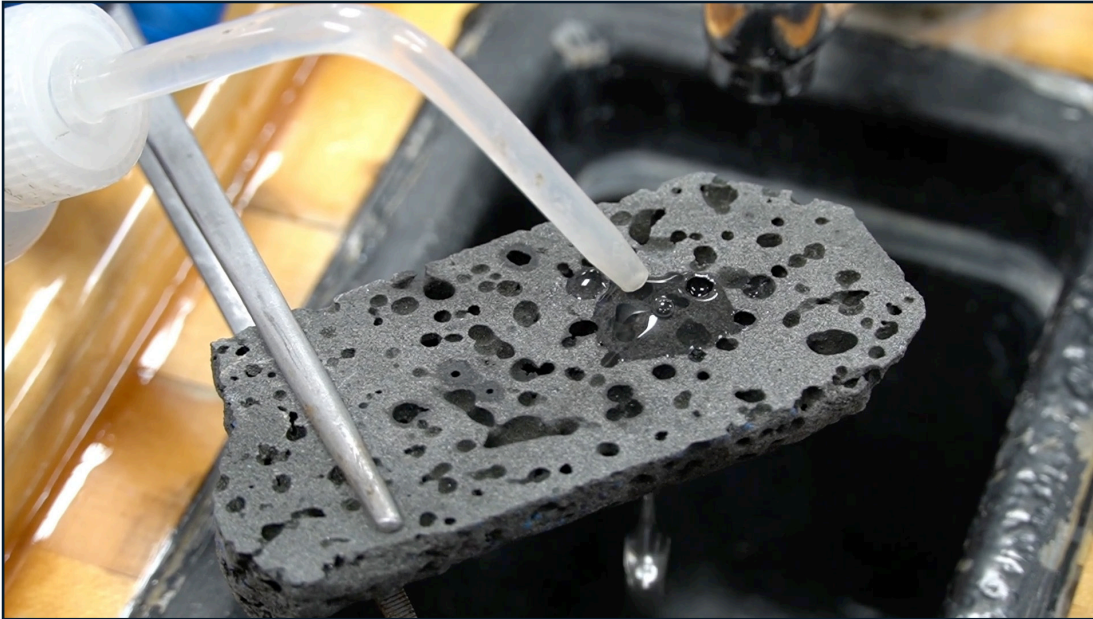
The rock from the upper layer of the flood basalts is so strongly permeated by vesicles that water quickly finds a way through.
