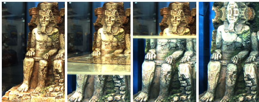
Figure 1: A model of the entrance to the Abu Simbel temple in Egypt is placed in a fish tank. A static camera views the scene through a flat glass. When increasing the water level in the fish tank, refractive effects are clearly visible. These do not only scale the image (in 2D) but allow to “look around” foreground objects (in 3D).
